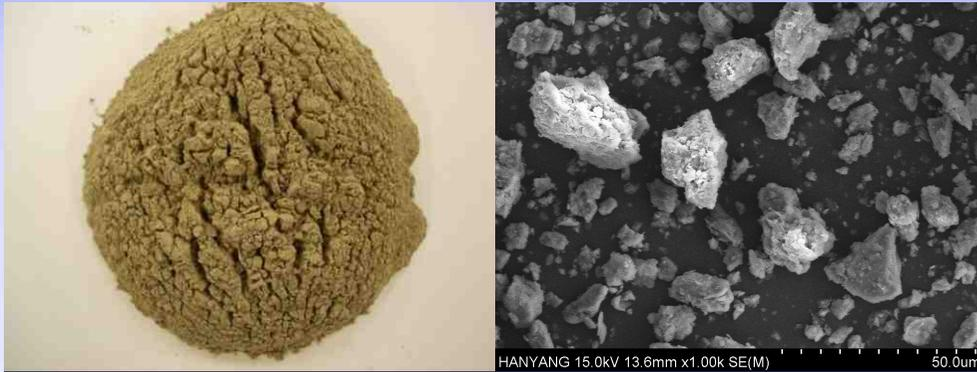
Lunar Simulant KOHLS-1(left) and SEM image(right)
