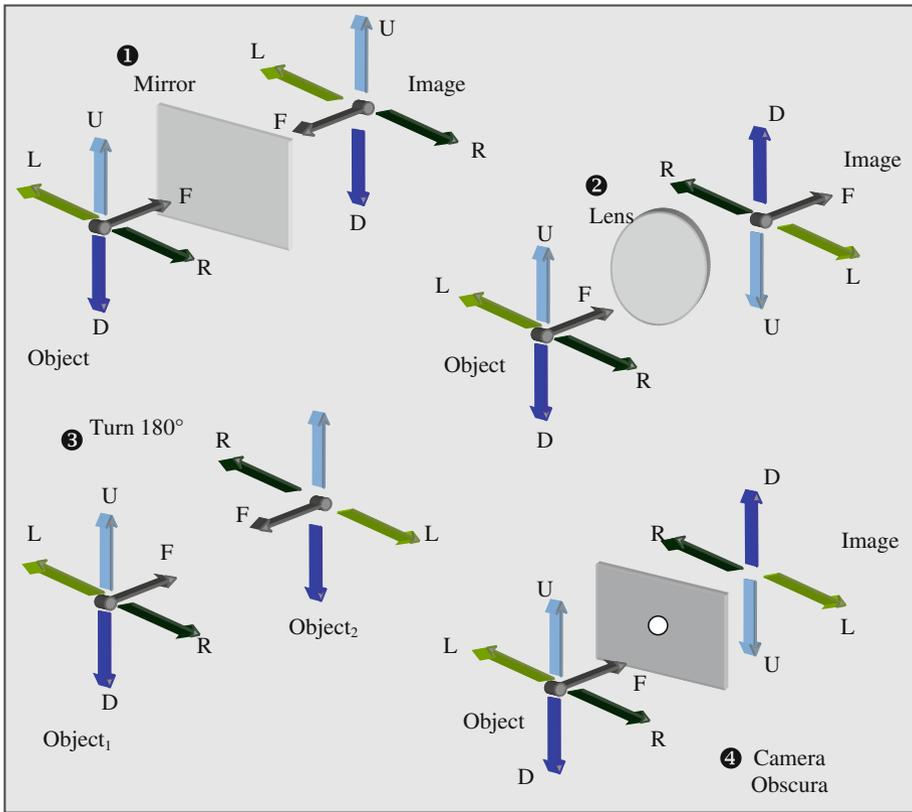
**Fig. 7** Transformation of object-image dimensions in four basic situations: 1 In the *plane mirror*; 2 In the real image by the *convex lens*; 3 When two persons face each other; and 4 In *Camera Obscura* (no depth of the image). To share the assumed considerations of Giotto compare cases 1 and 3
